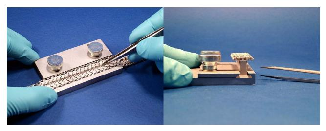
Use tweezers or holding stick to sort out the links, you can lock then prepared track length with sliding part secured with screws (for resin or plastic links you can now apply glue, its remains can be easily removed at the end from the metal surface)
