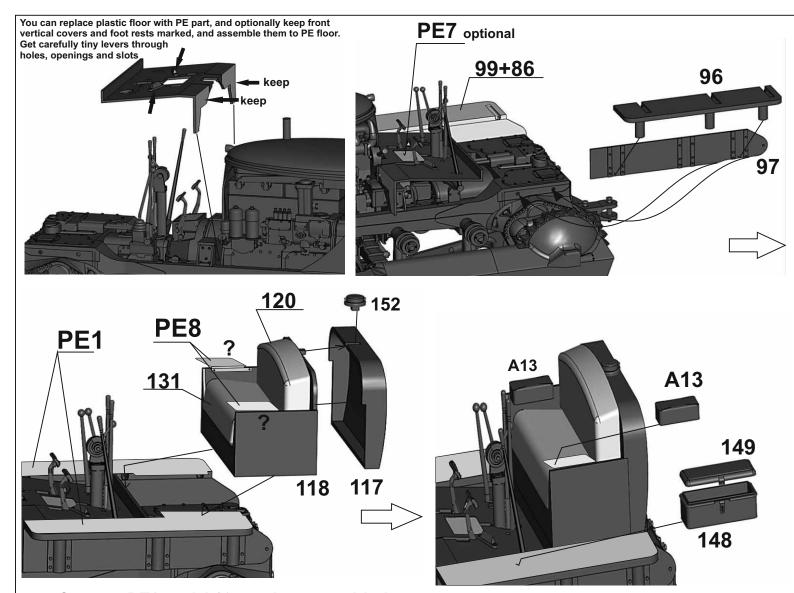
arm's rests PE8 and A13 can be assembled inside or outside the seat
