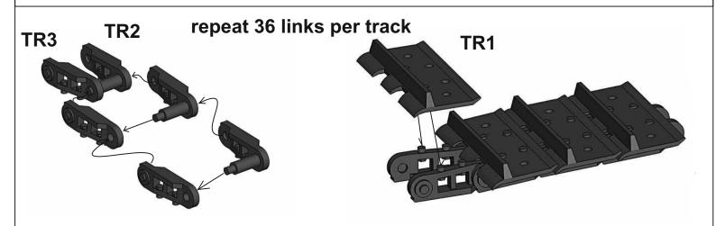
Mind correct direction of tracks! Track links are workable, however it is recommended to assemble them in short sections around, leaving the top for the end, and secure them with glue
