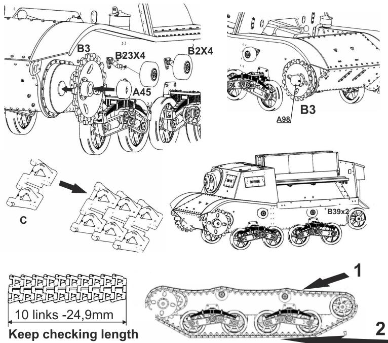
Keep checking length of the tracks during assembly, do not leave gaps between links
