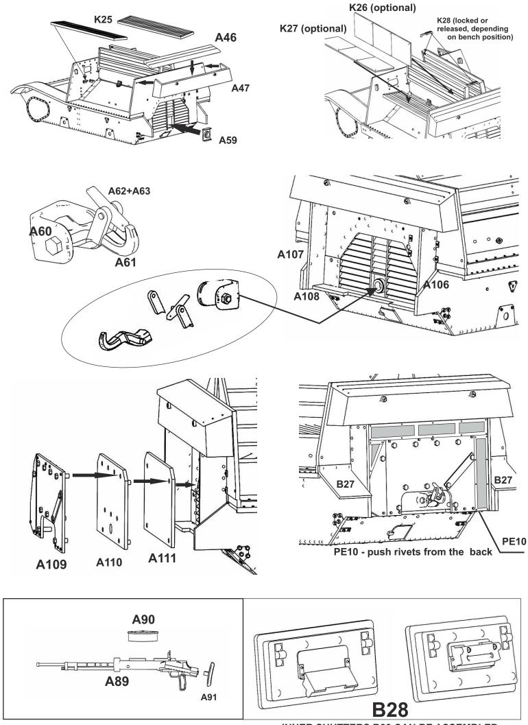
INNER SHUTTERS B28 CAN BE ASSEMBLED EITHER OPEN OR CLOSED
