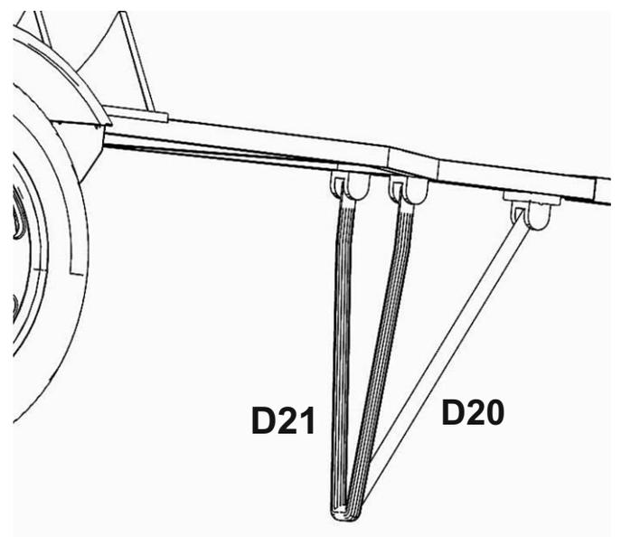
you can assemble holding legs either in standing or traveling position
