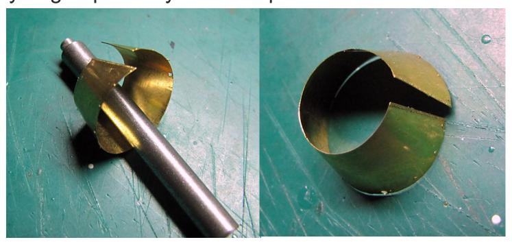
Plastic option because of injection molding limits regarding minimal wall thickness to fill the design properly looked strange, that we decided not to use it. The same for Bren gun assembly, it would be double thick than it is supposed to be.
