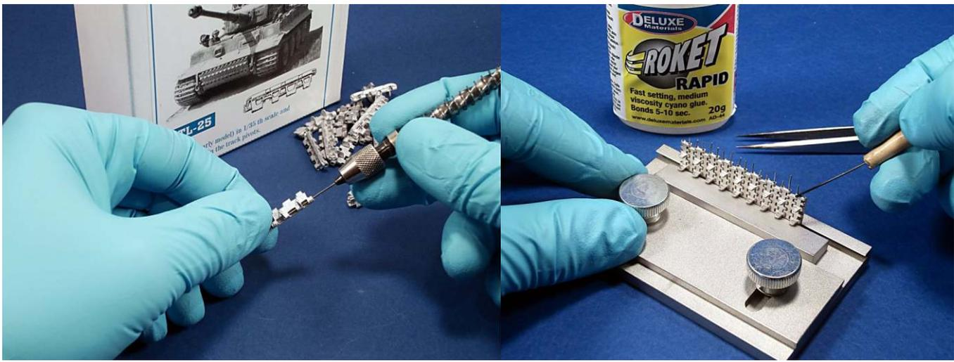
Place a metal pin in the holes and connect all the track links.
