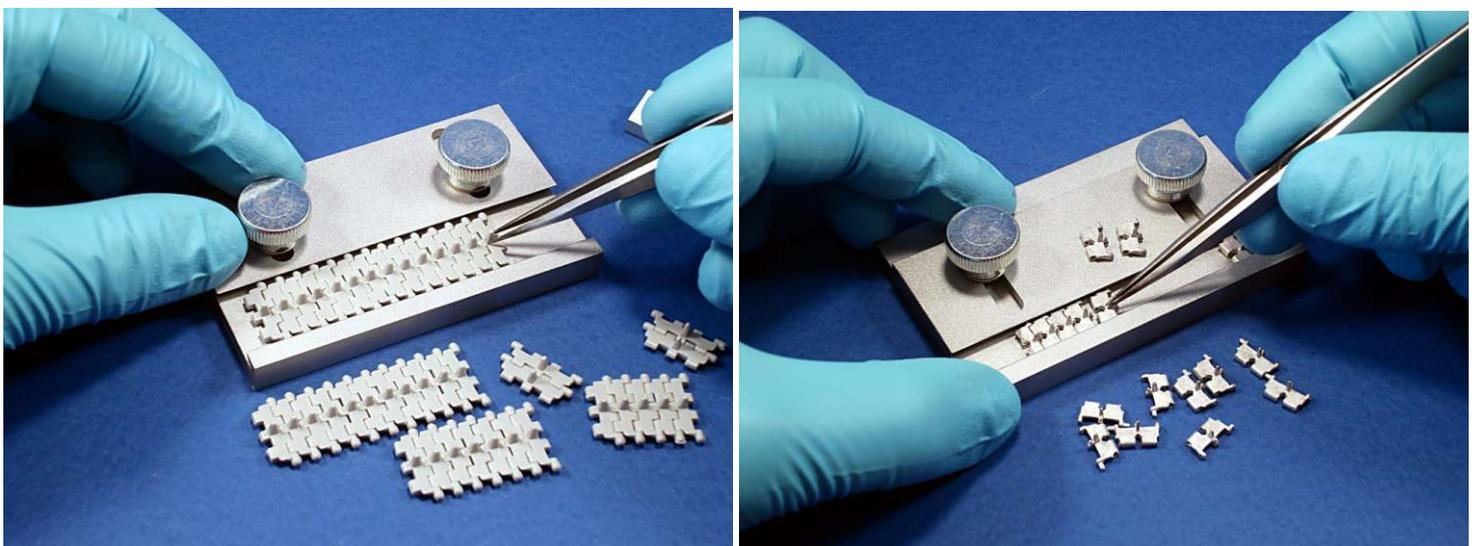
No matter if the track links are in plastic, metal or resin. The assembling process is always the same. Just prepare track links and get ready to assemble them.
